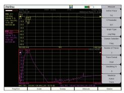
Cable & Antenna and VNA Mode in the LMR Master both provide simultaneous measurement of insertion loss and return loss  $% \left( {{{\rm{A}}_{{\rm{A}}}} \right)$
