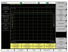
**RF Measurement – Average Burst Power** High or low values will create larger areas of cell-tocell interference and create lower data rates near cell edges. Low values create dropouts and dead zones.
